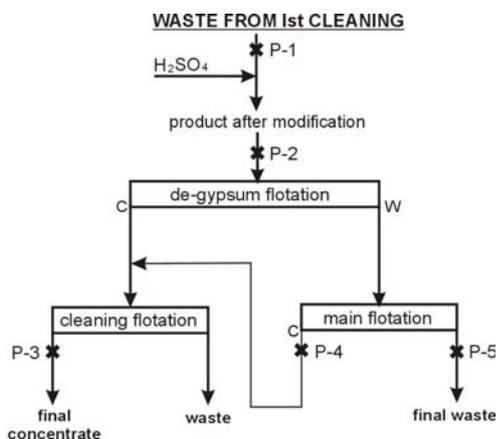
Figure 2. Diagram of enrichment with marked points of sample collection
