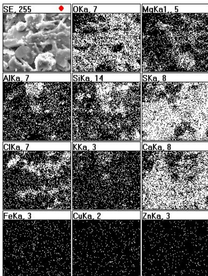
Figure 3. EDS map of particular elements distribution in the selected area of sample P-2
