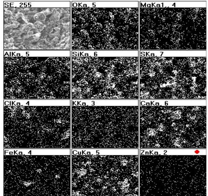
Figure 7. EDS map of particular elements distribution in the selected area of sample P-3
