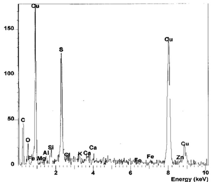
Figure 9. EDS plot showing the presence of particular elements distribution in an analyzed spot of sample P-3
