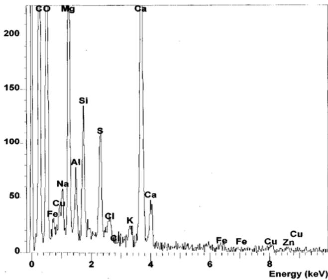
Figure 5. EDS plot showing the presence of particular elements distribution in an analyzed spot of sample P-2
