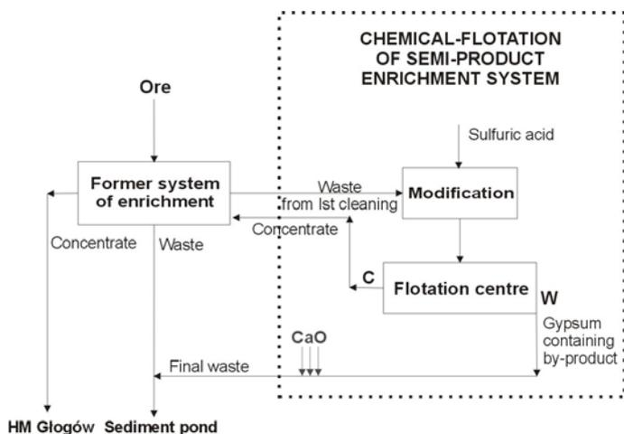
Figure 1. Block diagram of chemical – flotation enrichment technology
